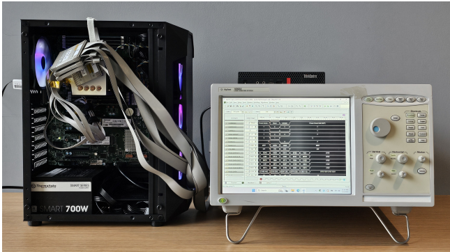
Figure 1: Our memory interposition setup, with target machine (left) and logic analyzer (right). Notice the gray wires from the DIMM interposer.
