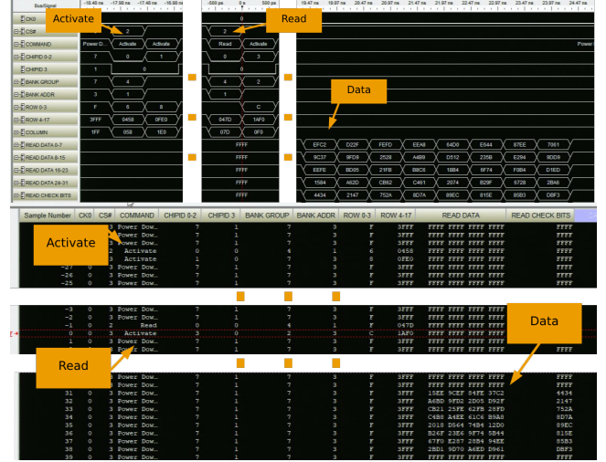
Figure 4: (top) A read command on the logic analyzer in the Waveform view. (bottom) A read command on the logic analyzer in the Listing view.
